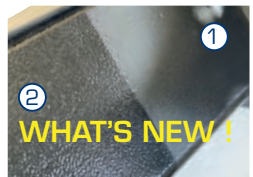
POWDER COATING PAINT (2) ADDED TO KTL PLUS (1). NO RUST AND NO SALT STAINS.
